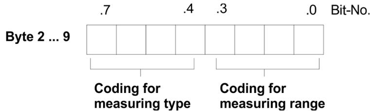
The corresponding codes can be found at parameterization of each module. The table is divided into measuring type like voltage, current, resistance measuring... Here the corresponding binary code of the measuring type may be found. Within the measuring types there are the measuring ranges, for which a binary measuring range code is to be specified in each case.
