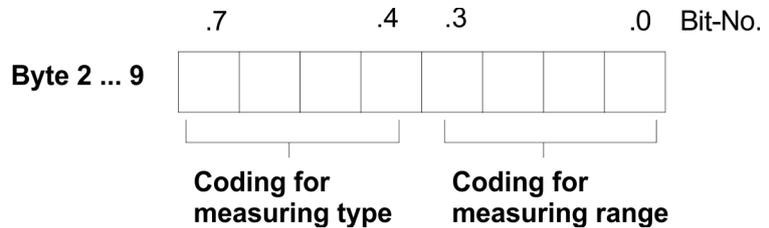
The following section shows an overview of all measuring types and ranges plus binary coding for the parameterization. Additionally, the wiring diagram assigned to the measuring range is shown in brackets.
