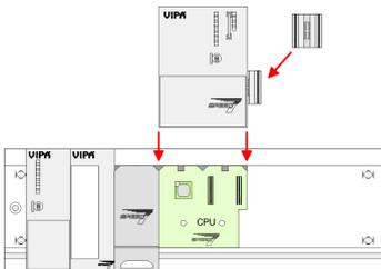
1. ➔ If also standard modules shall be plugged, take a bus coupler and click it at the CPU from behind like shown in the picture. Plug the CPU between the triangular positioning helps to the slot marked with "CPU SPEED7" and pull it down.
