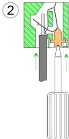
**2.** Insert the de-isolated wire into the round opening. You may use wires with a cross-section from 0.08mm<sup>2</sup> to 2.5mm<sup>2</sup>
