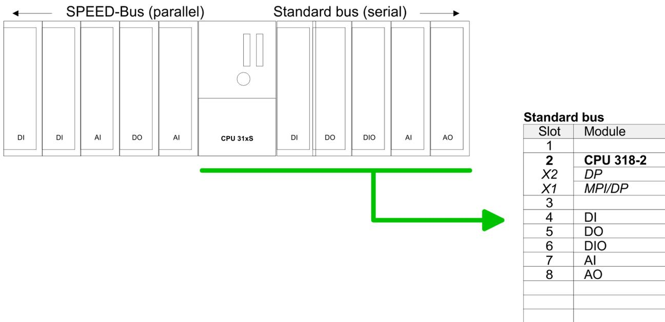
**i** To extend the bus you may use the IM 360 from Siemens where you can connect up to 3 further extension racks via the IM 361. Bus extensions are always placed at slot 3.
