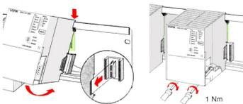
2. ➔ Plug the CPU between the triangular positioning helps to the plug-in location marked with "CPU SPEED7" and pull it down. Fix the CPU by screwing.
