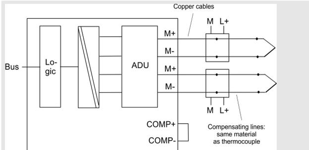
M+: measuring line (positive) COMP+: Compensation connection (positive)
