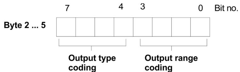
The corresponding codes can be found in the following table. Within the output types the output ranges are specified, for which a binary output range code is to be specified in each case.
