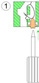
**1.** For cabling you push the locking vertical to the inside with a suitable screwdriver and hold the screwdriver in this position.
