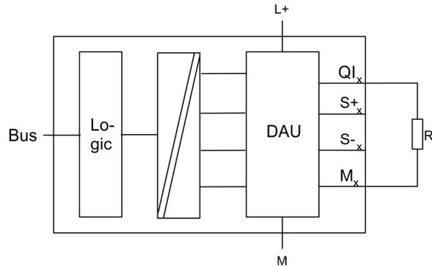
**Connecting loads at voltage output at 4-wire cabling (only 332-5Hx01)**
