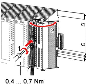
8. ▶ Bolt the fixing screw of the front connector.
