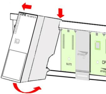
2. ▶ At deployment of a DC 24V power supply, install it at the shown position at the profile rail at the left side of the SPEED-Bus and push it to the left to the isolation bolt of the profile rail.
