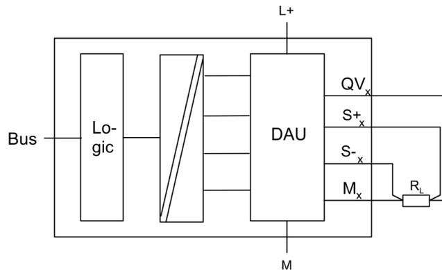
**Connecting loads at voltage output at 2-wire cabling**
