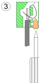
**3.** By removing the screwdriver the wire is connected safely with the plug connector via a spring.
