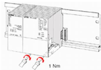
If you do not deploy SPEED-Bus modules, the assembly happens with the following approach:
