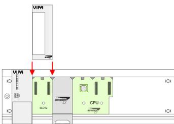
4. ▶ To connect the SPEED-Bus modules, plug it between the triangular positioning helps to a slot marked with "SLOT ..." and pull it down.
