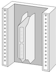
For the communication between the modules the System 300S uses a backplane bus connector. Backplane bus connectors are included in the delivering of the peripheral modules and are clipped at the module from the backside before installing it to the profile rail.
