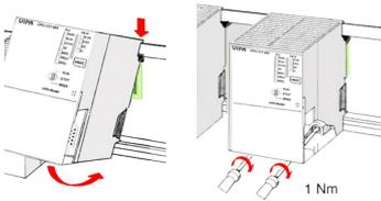
2. ➔ Fix the CPU by screwing.
