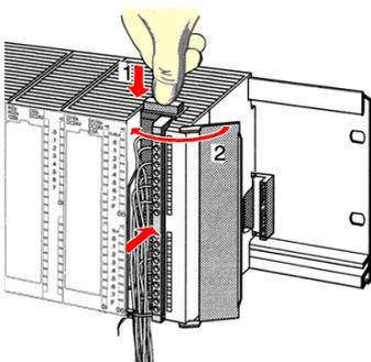
8. ▶ Push the release key at the front connector on the upper side of the module and at the same time push the front connector into the module until it locks.
