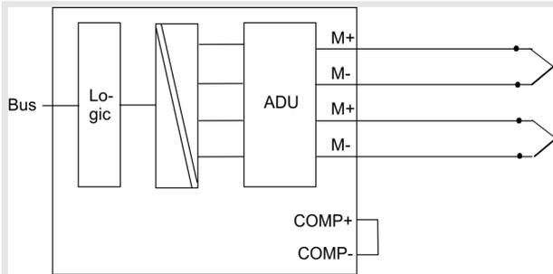
**Thermocouples without compensation slot and external compensation**
