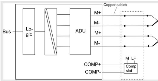
When connecting thermocouples with one compensation slot, you have to regard that the thermocouples have the same type. The compensation slot is to be connected at COMP+ and COMP- and is to be supplied external.
