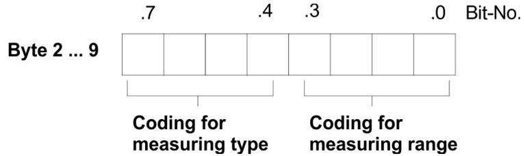
The following section shows an overview of all measuring types and ranges plus binary coding for the parameterization.
