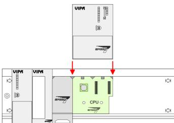
1. ▶ To deploy the SPEED7-CPU exclusively at the SPEED-Bus, plug it between the triangular positioning helps to the slot marked with "CPU SPEED7" and pull it down.
